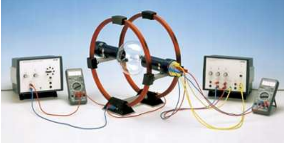
Fig. 1 Experimental set-up for determining the electron charge to mass quotient.
