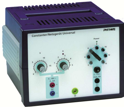
Fig. 5 Power supply for Helmholtz coils.
