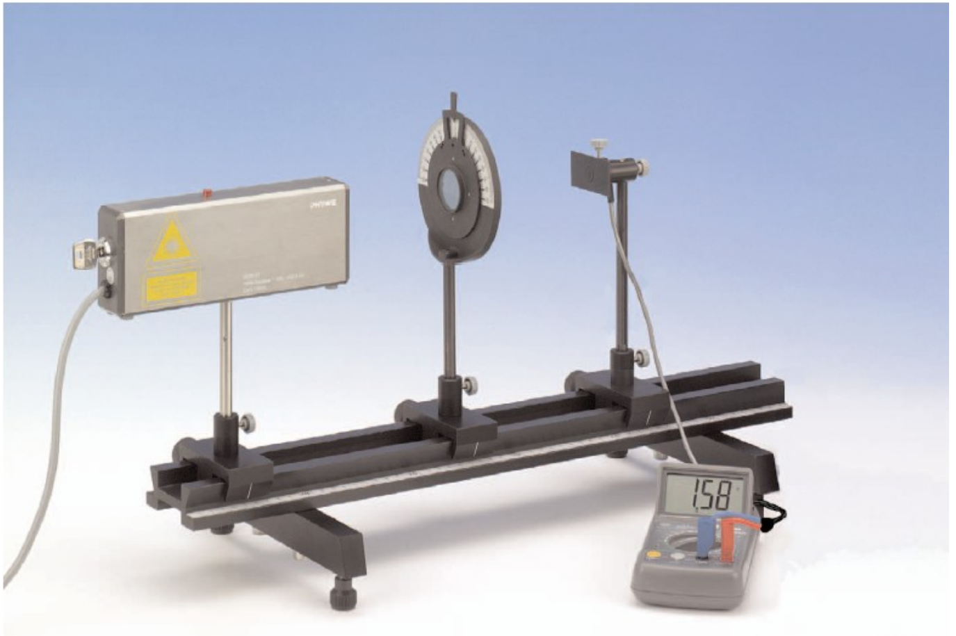
Fig. 1: Experimental set-up: Malus' law.
