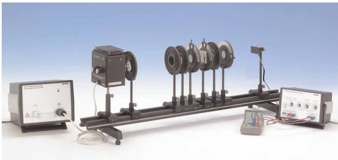
Fig. 1: Experimental set-up for determining the type of polarisation of the emergent light.
