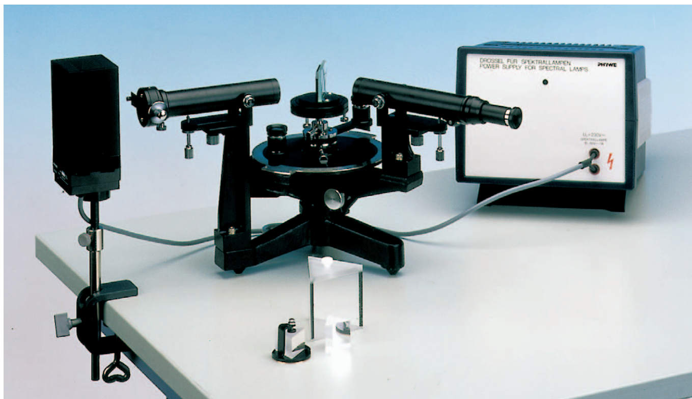
Fig. 1: Experimental set-up for determining dispersion in liquids.
