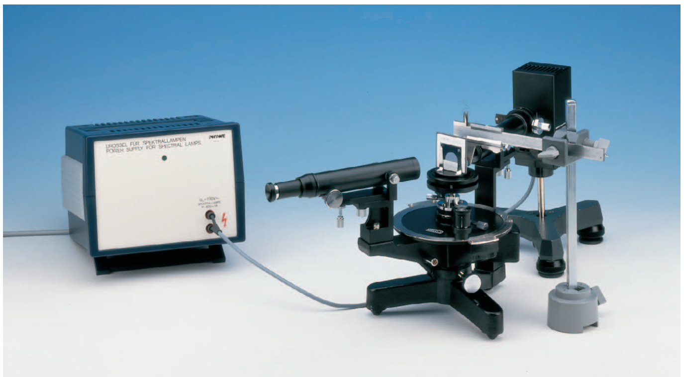
Fig. 3: Experimental set-up with vernier used as auxiliary slit to determine the resolving power.
