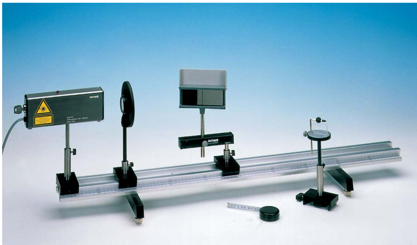
Fig. 1: Experimental set-up for producing interference with the Fresnel mirror.
