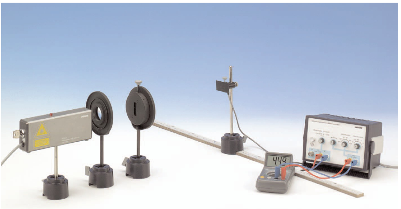
Fig 1: Experimental set-up for the diffraction of light at a slit and an edge.
