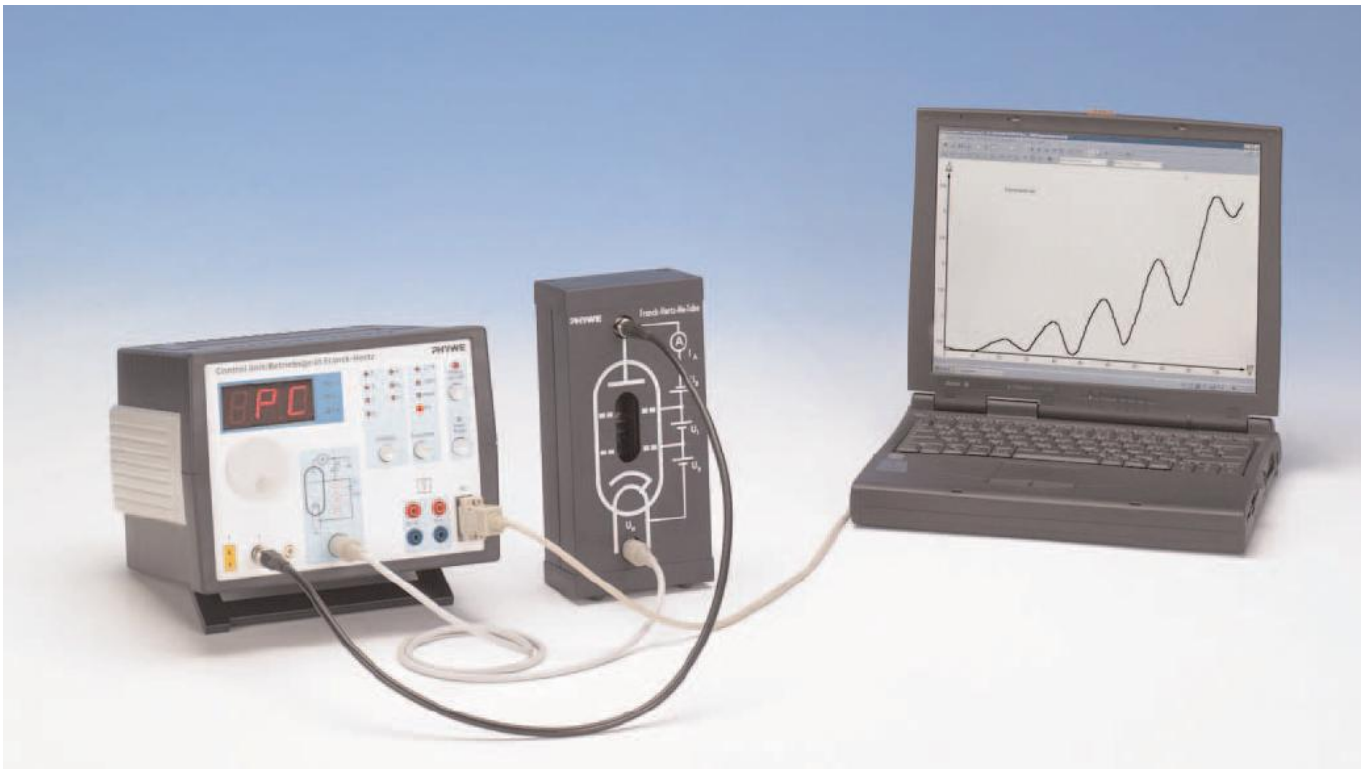
Fig.1: Set-up for the Franck-Hertz experiment with PC.
